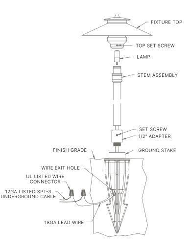
TIP: Small gauge cable is vulnerable to damage in the landscape; Protect by routing in close proximity to the luminaire or adjacent to concrete slab or similar structure. Do not bury more than 6" deep. Do not over tighten.
